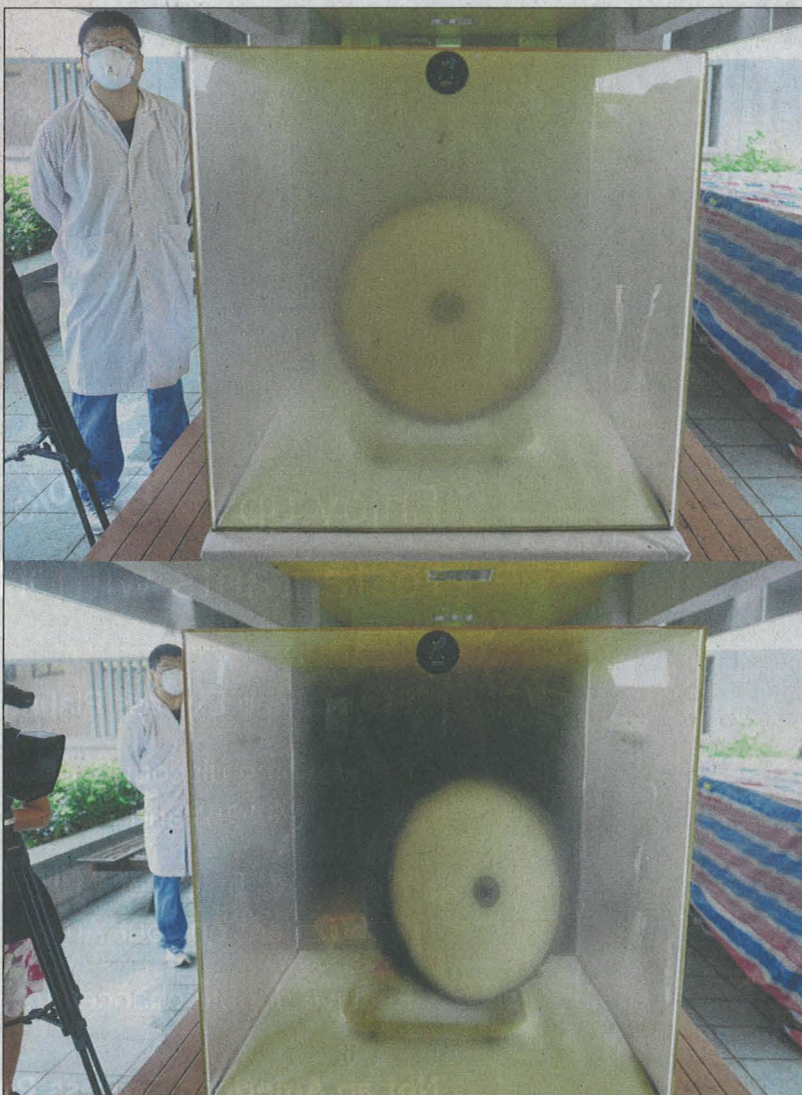
A fan fitted with one of the NUS filters clears the smoky air inside a box in these before (top) and after photographs. ST PHOTO: MARK CHEONG
